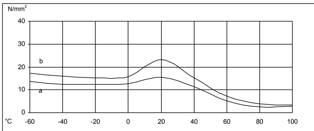
**Roller peel test (ISO 4578) (typical average values)**
