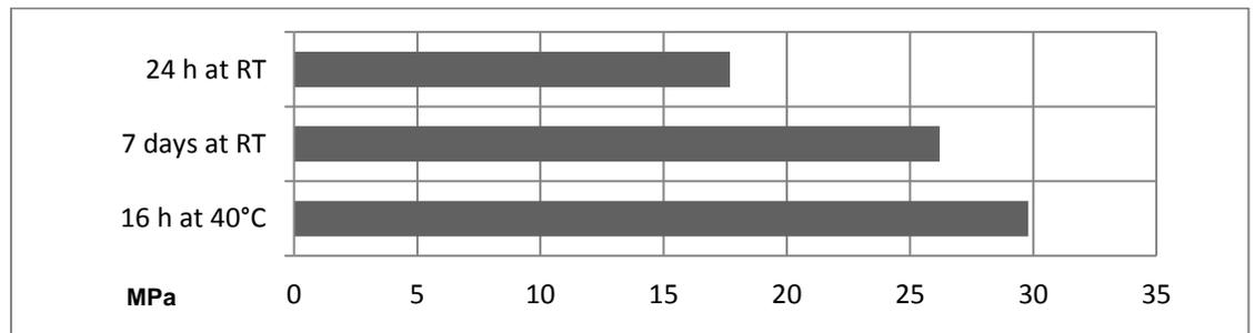
**Average lap shear strengths of typical plastic-to-plastic joints (ISO 4587) (typical average values)**
