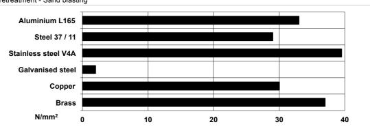
Cured for 7 days at 23°C and tested at 23°C Pretreatment - Sand blasting
