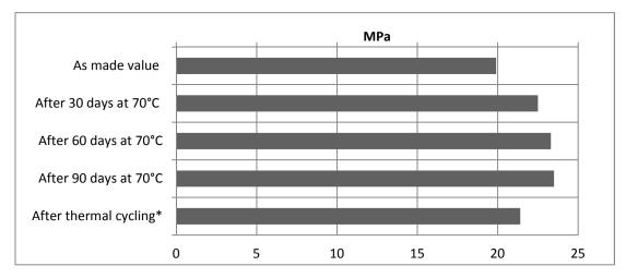
\* Thermal cycling: 25 cycles of 6 hours duration from -30°C to 70°C
