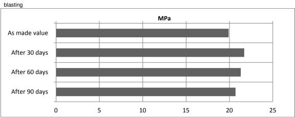
(40°C/92% Relative Humidity) On aluminium, cured for 16 hours at 40°C and tested at 23°C. Pretreatment - Sand blasting
