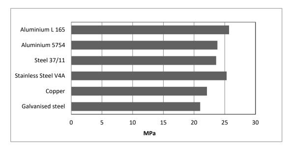
Average lap shear strengths of typical metal-to-metal joints (ISO 4587) (typical average values)
